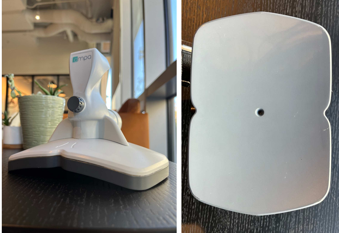
Figure S2. Treatment coil with integrated endoscope camera. The centrally-placed, 4 mm diameter endoscope camera on the underside of the coil enables accurate placement of the coil over the intended target, indicated on the cap with a pre-printed circle inscribed with an alphanumeric identifier.
